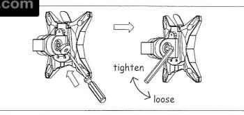
1. Use a flat-pin screw-driver to push open the plastic cap.
