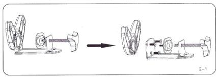
2.Re-install the base plate with three retained attach screws,tighten these screws with a 4mm allen key and paste the rubber pad on the one screw as shown on 2-2
