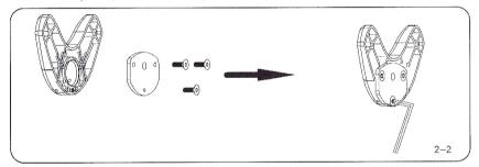
3.From below desk,insert retained clamp adjustment through pad and up through hole in desk,Thread screw by turning the knob into base plate but not tighten completely at this time,Center the desk mount assembly over hole,securely tighten screw as shown on 2-3
