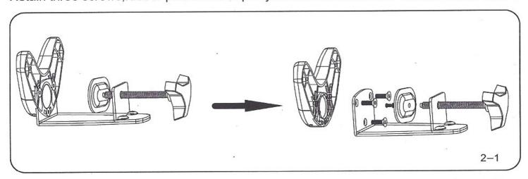
2.Re-install the base plate with three retained attach screws, tighten these screws with a 4mm allen key and paste the rubber pad on the one screw as shown on 2-2
