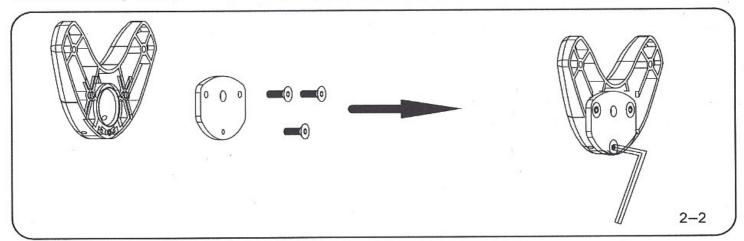
3.From below desk,insert retained clamp adjustment through pad and up through hole in desk,Thread screw by turning the knob into base plate but not tighten completely at this time,Center the desk mount assembly over hole,securely tighten screw as shown on 2-3
