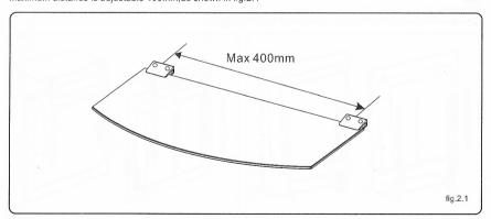
Assembled the glass panel mounted clamps and bracket
