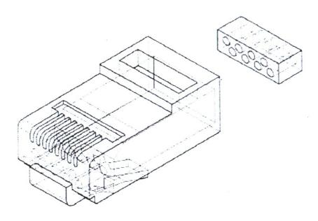
Figure D.11 - Example of a two-piece (insert) modular plug
