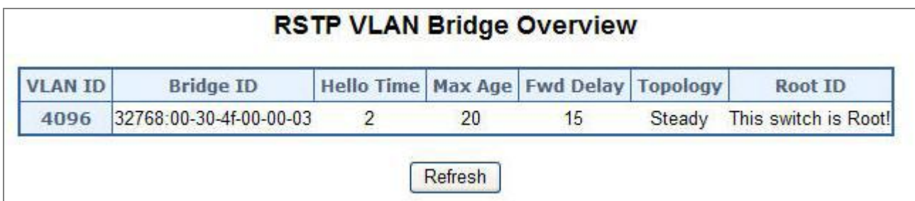
Figure 4-60 RSTP VLAN Bridge Overview
