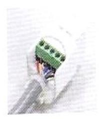
Use a screwdriver to tighten the wires onto the screw terminal.
