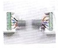
Arrange the wires and insert into the screw terminal block.
