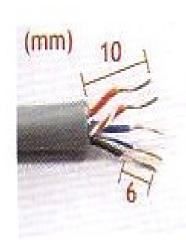
1. Strip the cable jacket length for about 10mm.
