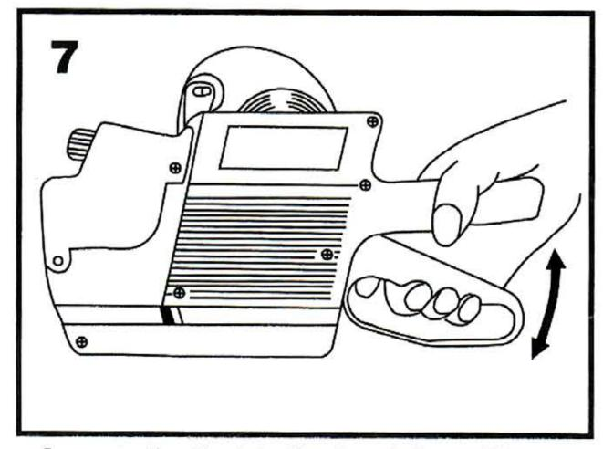
Operate the the labeller 2 or 3 times. Then the printing labels come—out.
