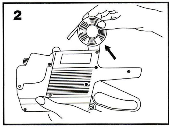
Return the label case to original position after inserting the label.
