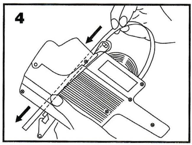
Insert the label to the direction of arrow sufficiently.
