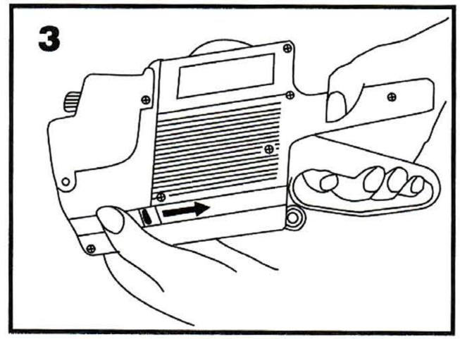
Press the base plate open key to the direction of handle. Then the base plate will be opened.
