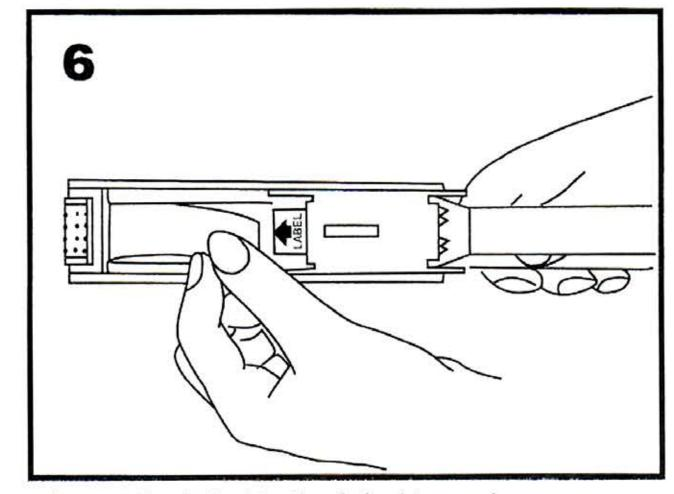
· Insert the label to the label tunnel.
