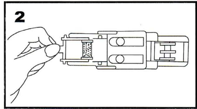
Insert the new Ink- Roller to case as per drawing and Re-Insert the Ink-Roller case to the machine.
