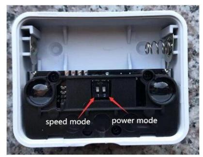
Transmitter 1# DIP switch slider to the ON end indicates high speed mode Transmitter 1# DIP switch slider to 1 end indicates low speed mode Transmitter 2# DIP switch slider to the ON end indicates high power mode Transmitter 2# DIP switch slider to 2 terminals to indicate low power mode
