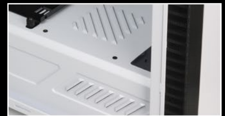
Air Vents for Optimal Cooling of Drives
