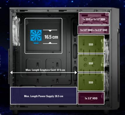
Apart from a drive bay for an optical drive, the VG6-W offers sufficient mounting options for data storage: Three 2.5" drives have space on the inside side panel behind the front fans. In the drive cage under the optical drive bay, a 3.5" and a 2.5" drive can be mounted. There is space for another 3.5" drive on the bottom panel below the fans. If an optical drive is not needed, its drive bay can be used for another 3.5" drive.
