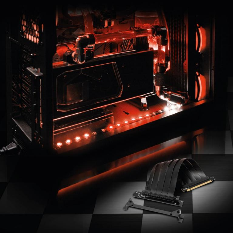
The Sharkoon Vertical Graphics Card Kit allows graphics cards to be vertically mounted quickly and easily. Illuminated graphics cards can thus be optimally presented from their best side! The installation kit was especially developed for the ELITE SHARK series and consists of a mount for the graphics card and an extra-long riser cable. The mount is simply screwed onto the power supply tunnel, and the riser cable is then connected to the mainboard and the graphics card.
