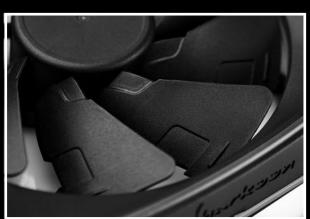
The RGB SHARK Lights are equipped with a newly developed type of aerodynamic blades and also possess a fluid dynamic bearing, all of which produces an air flow rate of 56 cubic meters per hour at 1,000 rpm and a quiet 15.2 dB(A).
