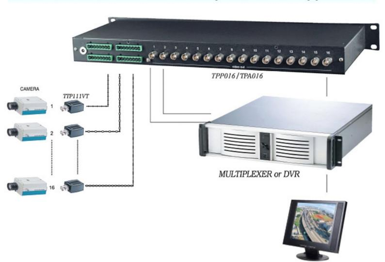
Using 8 or 16 receiver 1U panel on monitoring station, Professional 1U panel could reside in the same rack as other equipment, such as switcher, multiplexer, DVR...etc.
