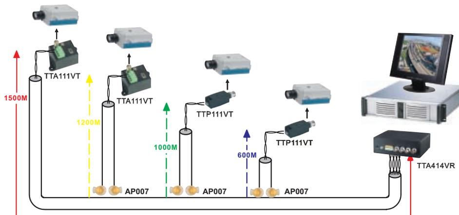
Passive or active video transceiver for series connection to use one CAT5 4 pairs cable, transmit 4 video signals for different range.
