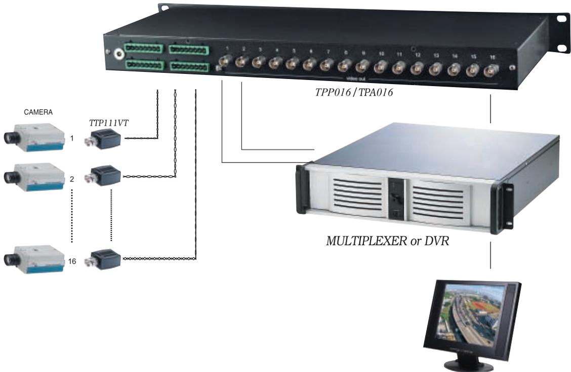
Using 8 or 16 receiver 1U panel on monitoring station, Professional 1U panel could reside in the same rack as other equipment, such as switcher, multiplexer, DVR...etc.
