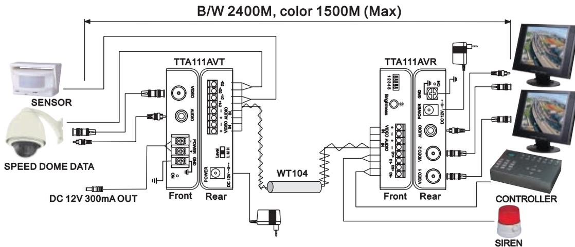
Using TTA111AV could transmit video, audio, 2 data signal, range up to 1.5KM (Color), 2.4Km (B/W)
