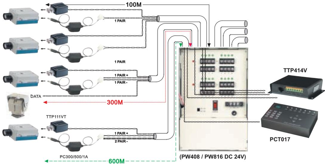
Using CAT 5 cable to transmit Video, Power, Data Signal for best & professional cabling management.
