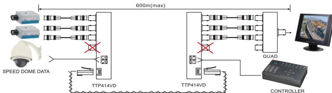
Using one 4 pair UTP cable to transmit/receive 4 sets video signals or use 3 pairs to transmit/receive 3 sets video signal, plus one data signal (RS422,485).
