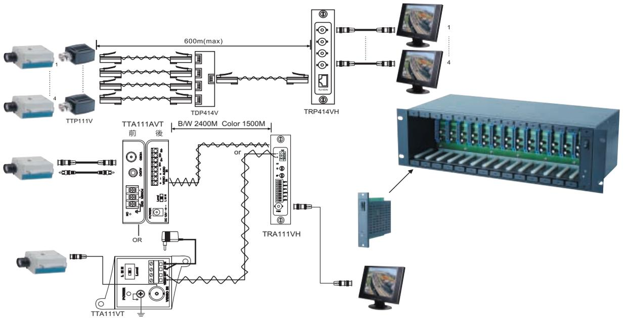
Using rack card type, could insert passive or active receiver card at TRN012 Rack Cabinet, the maximum receiving channel could up to 60 channels (passive).
