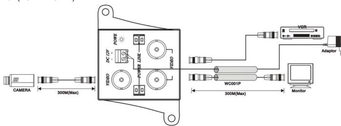
• When using multi distributors, a jumper is needed to extend power. (Max of 8 per power adapter) Package includes a jumper for power loop.
