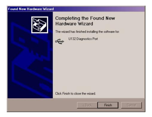
Because the U132 is a USB Composite Device, the "Found New Hardware" process will need to be performed twice. Again, when asked, do not allow connection to the Internet.
