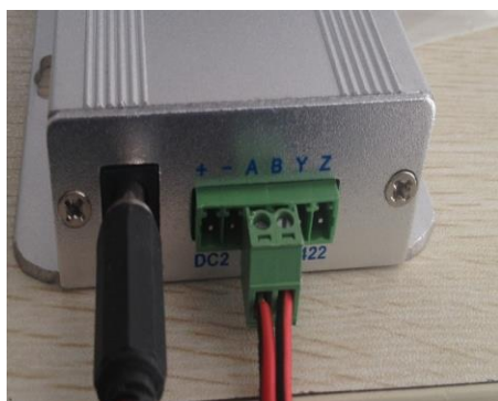
Power supply and RS485 interface
