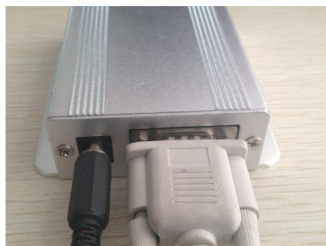
power supply and RS232 interface
