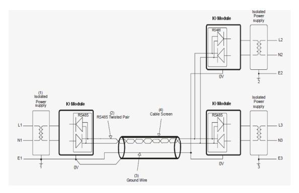
Note: Ground on IO module is Pin1 at 4 pin connector which is 0V or "-"V, Power supply
