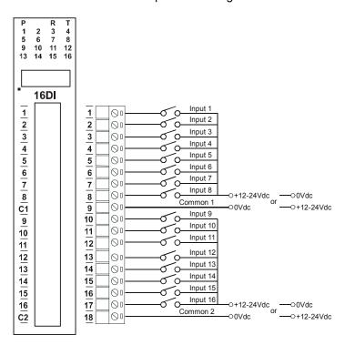
The following diagram shows how the digital inputs are connected a NPN transistor or a PNP transistor.
