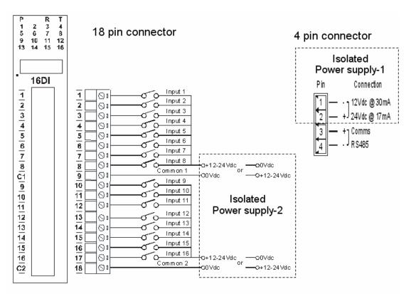
Note: Use separate isolated 24V DC power supply for Power supply and field inputs
