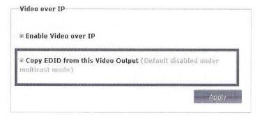
VKM03R Video over IP: This function setup the video signals send from network, select Copy EDID from this Video Output and enter "Apply" finish setting (pick up this item will auto copy VKM03R TV EDID).
