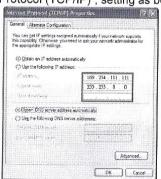
(IP address: 169.254.111.111 Submask: 255.255.0.0 Getway and DNS are not required)
