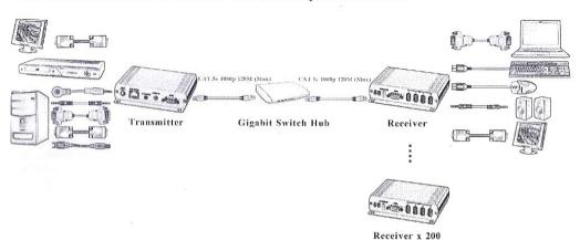
1 Input to Multiple outputs connections via a Gigabit network switch
