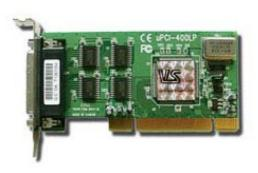
The Low Profile card fits to the PCI Low-Profile specifications. As such it is usable in small cases. The high speed serial ports with their long 128 byte FIFO are best for high speed communication, even in heavy loaded systems.
