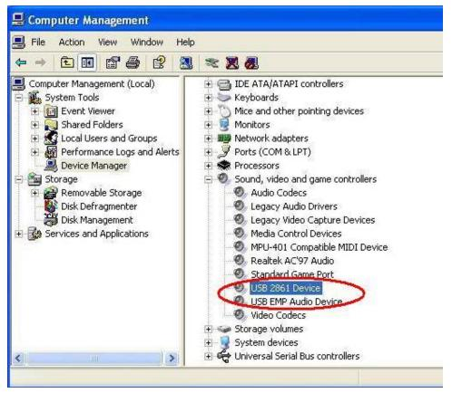
You can check the driver version for "USB 2861 Device" and "USB EMP Audio Device".
