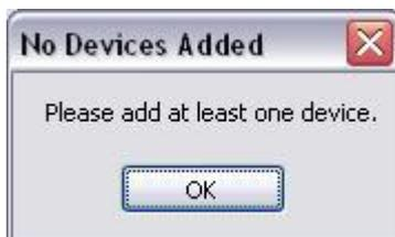
If after attempting to remove a device the application was unable to find any devices matching the Vendor ID and Product ID, the following message box will appear. In this situation make sure that the details that you have entered are indeed correct by checking with the windows device manager.
