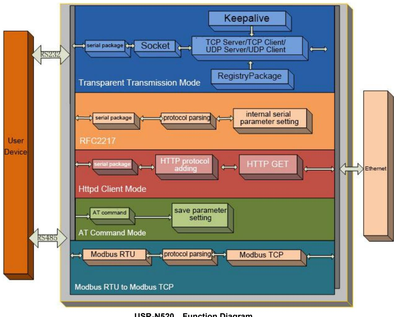
Each serial port corresponds to two socket: socket A and socket B. Socket B can be opened or closed.
