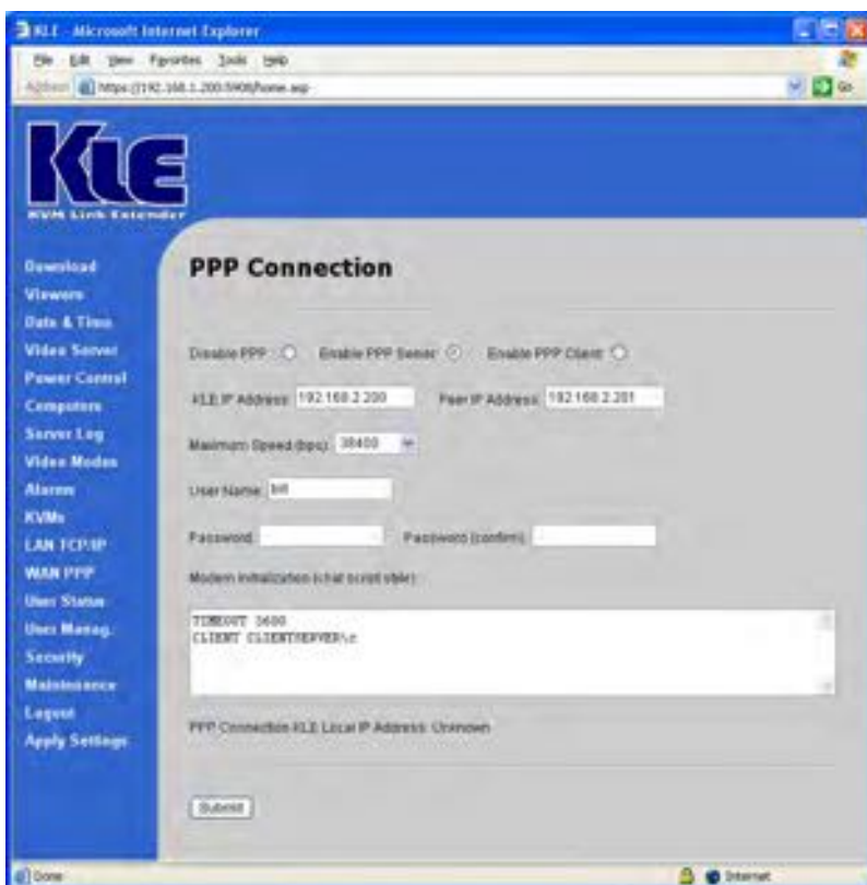
PPP Connection over direct serial cable with KLE as PPP Server
