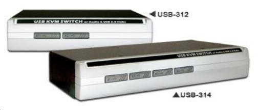
and a set of speakers and microphone. You can select the computers, USB device hub port control and audio/mic channel independently, using either front-panel buttons or keyboard hotkeys.
