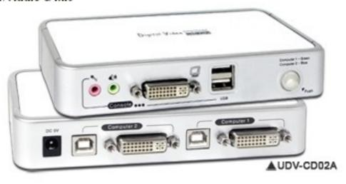
using the Switching Software Client installed on your PCs. It comes with 2 sets of detachable DVI/Audio&Mic combo cables & 2 USB cables for SOHO and office desktop multimedia application.
