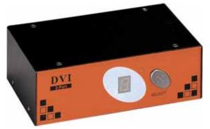
The UDV-002 DVI KVM Switch is designed specifically for sharing a DVI Monitor/Flat Panel Display between two DVIenabled PCs. You can use it to control two DVI-enabled PCs using only one keyboard, mouse and DVI monitor/Flat Panel Display.
