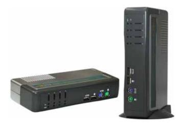
The UN72 is a 4-port USB PS/2 KVM Switch with Audio and Microphone switching function. It allows you to control 4 USB-enabled multimedia computers using only one PS/2 (or USB) keyboard, mouse, monitor and a set of speakers and microphone.
