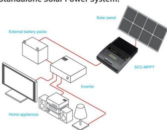
Combined MPPT technology and DSP controller, SCC-MPPT will convert best voltage to charge battery based on varied temperature. Compared to traditional solar charge controller, it allows your solar panels to operate at their optimum power output voltage, providing higher efficiency up to 98% with lower power loss.
