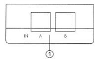
① TOSLink (Optical Fiber) Input Ports A and B: Connect the TOSLink input ports to the TOSLink output port of audio equipments such as audio amplifier, AV receiver or DVD player.
