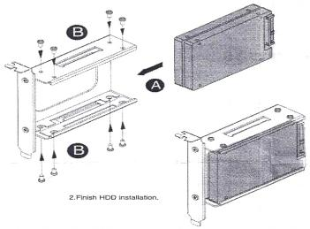
2. Lock HDD PCI frame with the screw, fix the HDD PCI frame on the host ,and cover the shell
