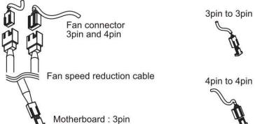
Fan speed reduction cable and installation specification.
