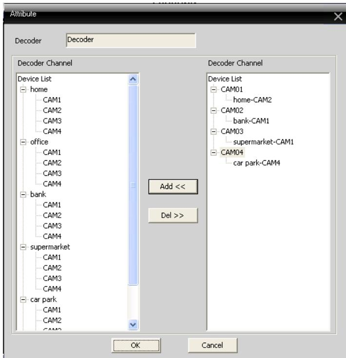
In the device list of left side,select 1 camera,then select 1 camera of right side,at last click "Add" in the center,for example:
