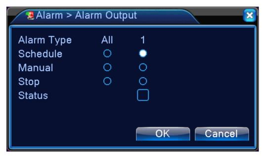
Please check current channel status: "o" means it is not in alarming status, "●" means it is in alarming status.
