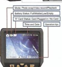
Insert card: Power off the device, open the cover on the backside of the monitor and insert the TF card according to this chart.
