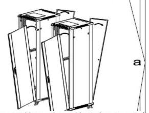
Remove side panels on sides to be connected
