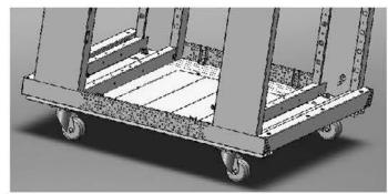
【1】: Use M8\*12 screws & M8 nuts to connect the frames, top & bottom. Note A: ensure the frame with earthing kits is at the right side, earthing kits is at bottom when assemble. B: Ensure the fan-unit at top & cable entry at bottom is close to the rear side.
