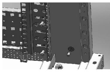
【6】: install the mounting rails. For 800mm width cabinet, install mounting rails to spacers by 2pcs of M6\*12 screws & M6 nuts. Check the picture in Step 5.
