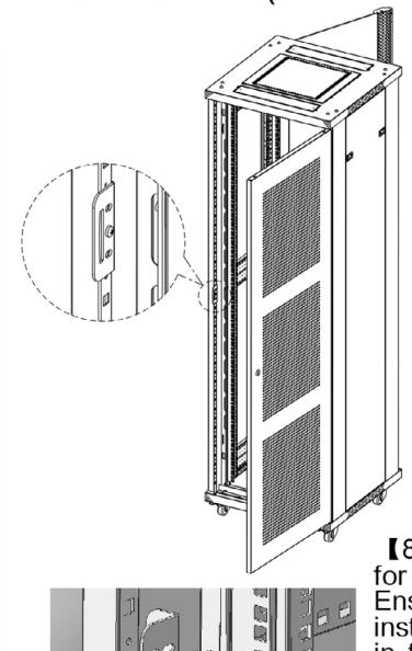
【8】: install the panel for lock. Ensure the panel installed to the frame is
