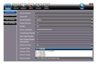
Systerm version: check the system version and time, when do software update, need to check version first to avoid updating failure and damage the device.
