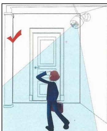
When people transversely across PIR detection area as to above picture, the camera will detect the movement sooner.
