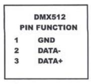
If you are using controllers with occupation, you can connect the DMX-output of the controller directly with the DMX-input of the first fixture in the DMX-chain. If you wish to connect DMX-controllers with other XLR-outputs, you need to use adapter-cables.
