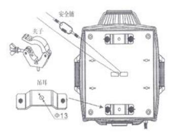
The strand wire is usually used in the shelf for the safety, the strand wire should stand ten times weiht than the machine, you should use the stand wire which has safety lock pins, the strand wire pass through the hole at the bottom, then tie it to the fixity, then tighten it.
