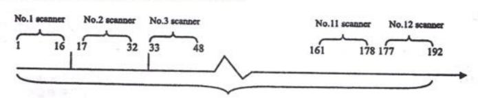
12 scanners, each is assigned 16 channels
