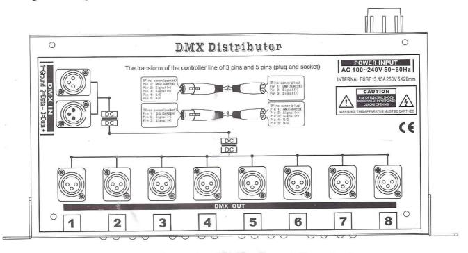
DMX input: from the DMX transmitting device DMX output: connect to the DMX receiving device
