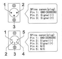
connector pin designations shall be as follows pin1:signal common(shield)
