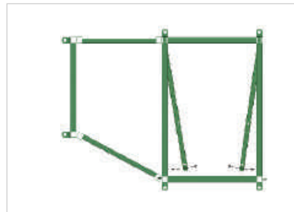
ONE-WAY SORTING ALLEY 90° [NDSA] WEIGHT: 521 lbs. DIMENSIONS: 70" w x 82" h x 54" l
