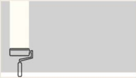
1. Apply adhesive on base surface
