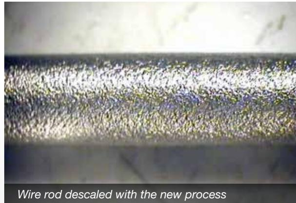
*Wire rod descaled with the new process*
