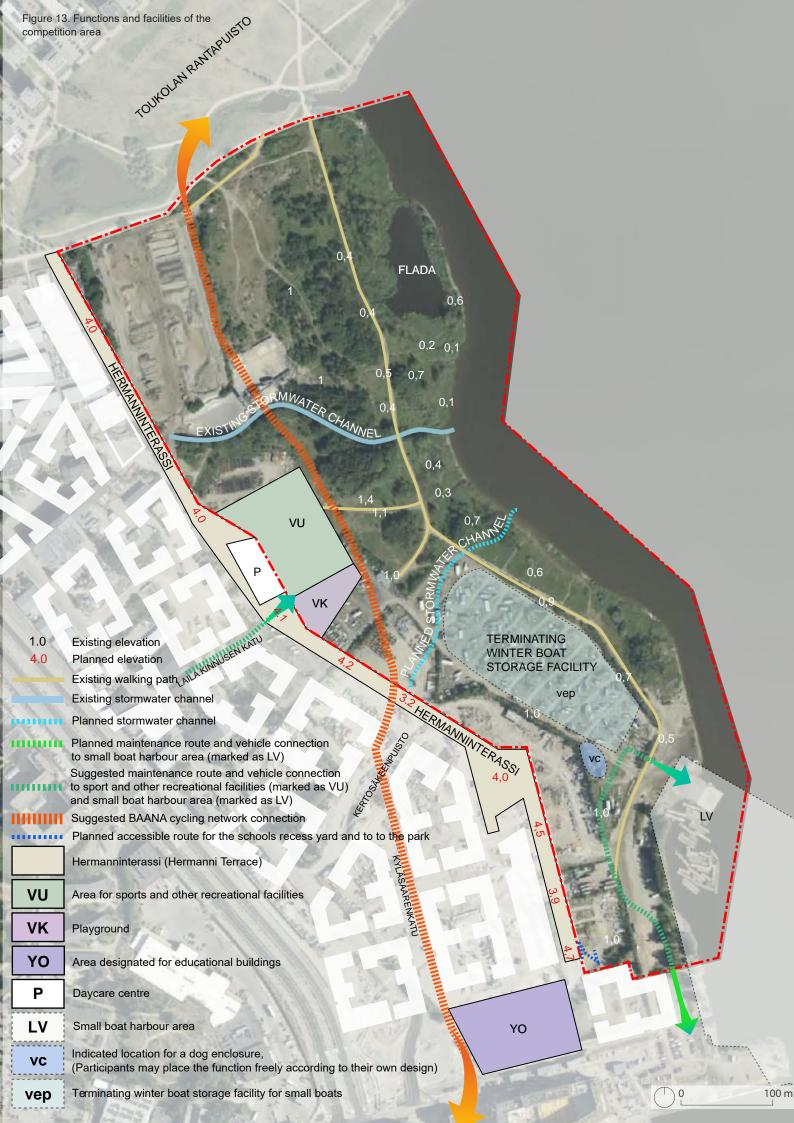
ally, because of the park's elevation, the Baana may be submerged during flood peaks. Nevertheless, solutions should be sought so that the Baana remains above water under normal conditions and is maintainable throughout the year.
