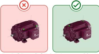
Installation on cooling fins and covers is not recommended.
