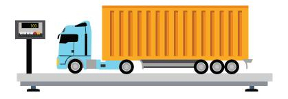
A. You may weigh the entire container, using calibrated and certified equipment. Then, subtract the weight of the container to get the gross weight of the cargo inside.
